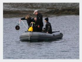
conventional deployment will be required. Highlight how the GPS reading will be taken and the need to reduce the distance between the shotline launch position and the GPS receiver to confirm accuracy.
