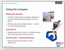
Bearing set using rotating bezel and cursors to north seeking needle
