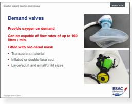
Just like on a SCUBA unit, demand valves supply oxygen only when the casualty breathes in (i.e. demands oxygen). The flow stops when the casualty stops inhaling. When they exhale, their expired gas escapes through a non-return valve into the surrounding environment.
